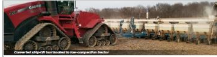
Converted strip-till tool loaded to low-compaction tractor
